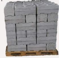
Cure blocks for 28 days before using in construction.
