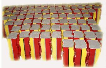
Moulds need to be stored on a level surface for 2 nights. The moulds must not be moved during this time as microscopic cracks will form decreasing the strength of the block. Put oil on top of blocks 30 minutes after casting to stop evaporation and cover with plastic sail.
