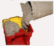
C: Do not top up the mould with mixture after casting, settlement of the mix is essential: 1 - 3mm. Do not fill the mould to the top,
